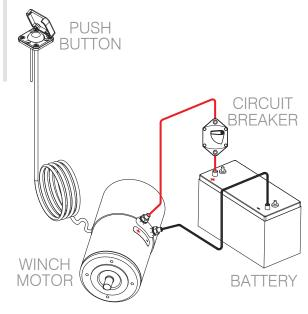
Motor units are supplied with installation manual, push button and cable terminals. Circuit breaker available separately. See motor unit product manual for push button to motor unit cable connection details.
