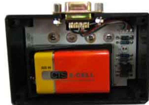
TS1-PK with 9V Battery installed
